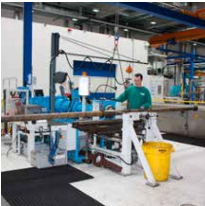
Extruder with stator for oil production
