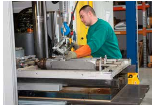
Injection molding machine for iFD-stators®
